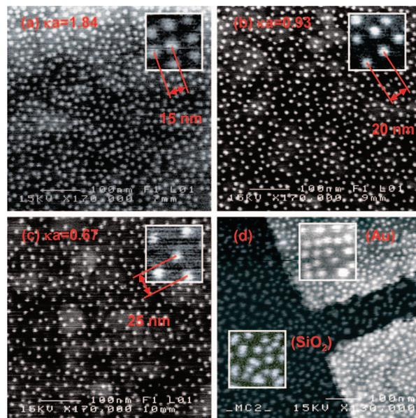
**Figure 2.** (a–c) Scanning electron microscopy pictures of octanedithiol modified gold surfaces with gold nanoparticles immobilized from citrate buffered solutions with decreasing ionic strength. (d) Gold nanoparticles adsorbed to a silicon substrate with gold patches modified with mercaptopropyl trimethoxy silane and octanedithiol respectively.
