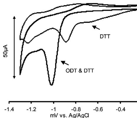
**Figure 1.** Cyclic voltammogram, first reductive sweep from 0 to  $-1.3$  V vs Ag/AgCl on gold surfaces modified with octanedithiol (ODT) and subsequently reacted with dithiothreitol (DTT) and reference surfaces modified with DTT only. The voltammogram was obtained in 100 mM KOH at a sweep rate of 200 mV/s.
